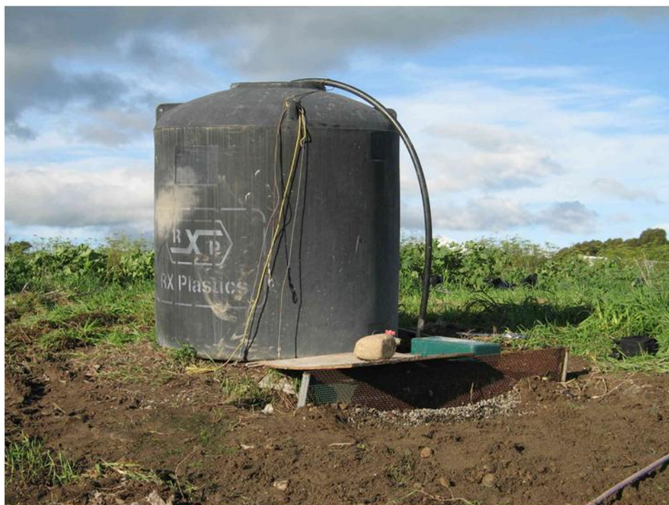
Figure 14 Header tank for dose loading of viruses
